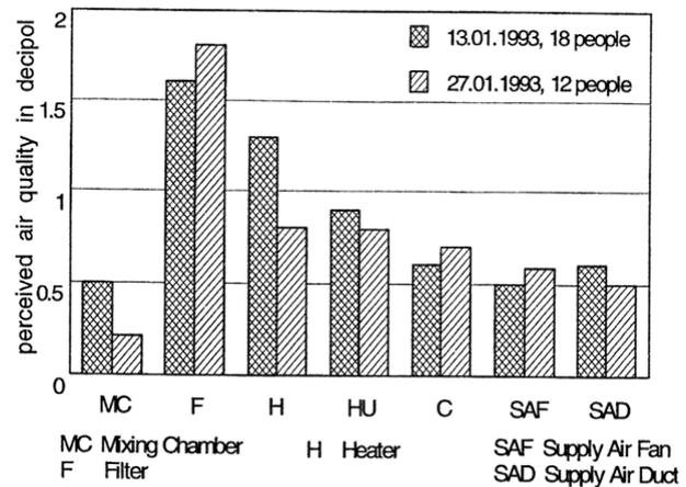
This sounds not logical because a filter reduces the amount of particles passing through, so how is this possible? There are both biological and chemical hypothesis stating that mechanical filtration is from biological perspective a placebo because it provides a “catch”-guarantee where a “kill”-guarantee is demanded. Consequences are:
