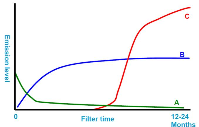
**Scientific research proofed that the introduction of technical measurements for improving IAQ (Indoor Air Quality) caused PAQ (Perceived Air Quality) issues due to emission of VOC's from caught micro organism on a filter bed. These issues can influence sick leave and productivity significantly.**
